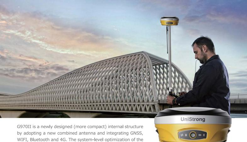
by adopting a new combined antenna and integrating GNSS, WIFI, Bluetooth and 4G. The system-level optimization of the whole machine brings a purer internal electromagnetic environment and better signal performance. The main body is made of pure magnesium alloy and has better electromagnetic shielding performance and a lighter and stronger body, which ensures stable and reliable operation and use of the equipment.
