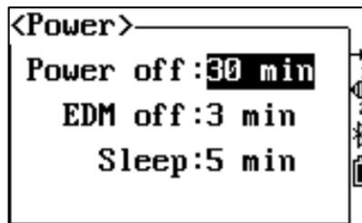
In default, the equipment will shut down automatically if there is no operation in 30 minutes.
