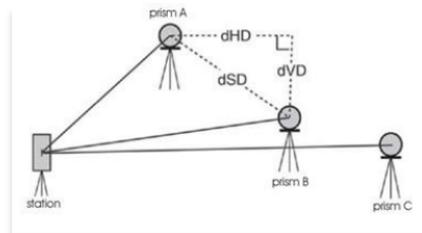
Press **[3] MLM Radial** to enter the function of MLM A-B, A-C <sup>PIC(1)</sup>.
