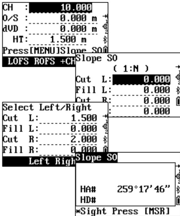
Input the ratio of left & right slopes to be cut or filled. Then select the slope in left or right side to staked out.
