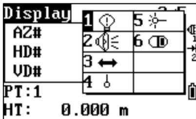
Press the key
