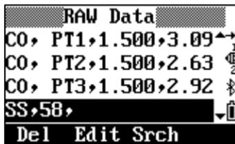
Hold 6.[DAT] for one second to change the type of data list (when press the 6.DAT).
