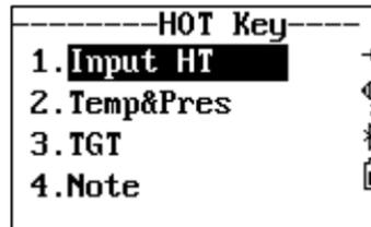
Press **[HOT./-+]** key, use **[▲]** or **[▼]** to move to the cursor or press the numeric key directly to choose the menu.
