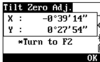
*Note: Please adjust the plate vial before the tilt sensor..*
