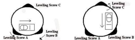
If the laser dot doesn't stay at the center position, please slightly loosen the screw under the tripod head and move the instrument (don't rotate the instrument) until the laser dot is on the station point. Tighten the screw and level the instrument again. Repeat these steps until the instrument is precisely centered and leveled.
