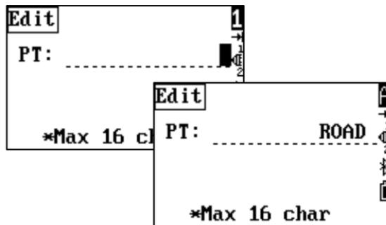
When **A** is shown on the screen, you can input alphabets; When **1** is displayed, numbers can be input.
