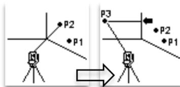
Press **[6] Corner Pt** to enter the corner point function <sup>PIC(1)</sup>.
