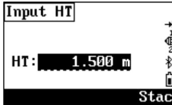
Enter the target height by manual; or press **F4 [Stac]** to select from stack. The HT Stack stores the last 20 entered HT values.
